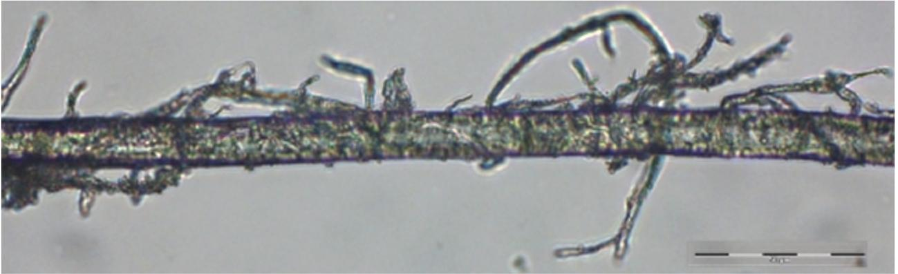
Fig 1. Frayed part of fiber; bf, scale bar 50µm
