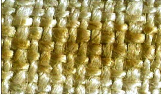
Fig. 3. (Color online) Photomicrograph of the cloth irradiated with 100 XeCl laser pulses. Intensity (fluence) = 16 MW/cm<sup>2</sup> (0.5 J/cm<sup>2</sup>) per pulse.
